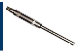
Total cell density (TCD) measurement by the Dencytee Arc sensor is based on the optical density or turbidity derived from a transmission and reflection signal at NIR wavelengths. The signal can be correlated with off-line measurements to achieve higher accuracy.
