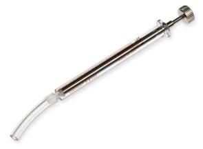
Pipette Controllers are intended to be used in place of rubber bulbs to easily and precisely fill glass pipettes. The free-sliding plunger coarsely fills the pipette, and the knurled plunger screw completes fine volume adjustment.
