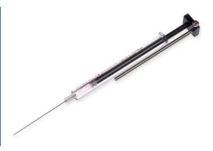
The Built-in Chaney adapter comes with a syringe installed from the factory. This eliminates the assembly step which can lead to damage of the smaller volume syringes. This is especially critical for 7000 series syringes which have extremely small plunger wires.
