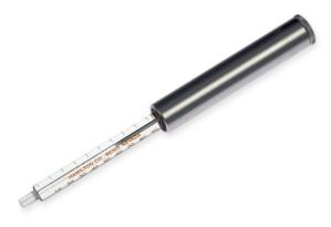
Threaded Plunger Syringes are for applications requiring extremely precise plunger movement or minute fluid manipulation. You can dispense from 0.33 to 37.79  $\mu$ L per plunger revolution depending on the syringe volume.
