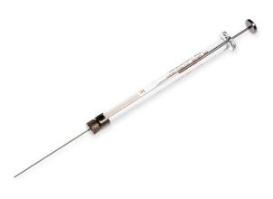
Hamilton Company's 600 series line of syringes are extremely low volume line of syringes. The 600 series syringes are similar to the 700 series only with half the stroke length and a reinforced stainless steel plunger.
