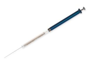
Split/splitless injection consists of a heated chamber with a glass liner into which the sample is injected through the septum. A microsyringe is used to inject the sample through a rubber septum into a flash vaporizer chamber at the head of the column.
