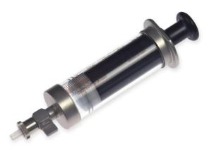
These Hamilton Gastight syringes are ideal for Purge and Trap applications because you can easily remove the syringe plunger and load water samples into the syringe barrel. You can add an internal standard or surrogate sample directly to your sample through the twist valve with a 10  $\mu$ L syringe.
