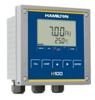
A traditional transmitter for pH, ORP, polarographic DO, and 2/4-pole conductivity. The H100 is a 4-wire design with dual 4-20 mA analog outputs and a relay for rinse and alarm functionality.
