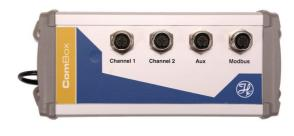
The Cell Density ComBox is a 2-channel USB device that enables the connection of two cell density sensors to the USB port of a Windows PC. The user provided PC must be compatible with the Hamilton cell density software.
