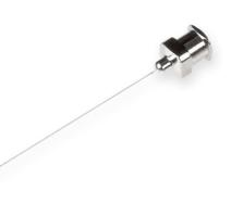
Metal (N) hub needles (nickel plated brass) are compatible with PTFE Luer Lock (TLL) syringes and plastic Luer Tip (LT) or Luer Lock (TLL) connectors. These 304 stainless steel needles are packaged in convenient 6 packs and are available from 10-30 gauge. Custom needle lengths and point styles are available.
