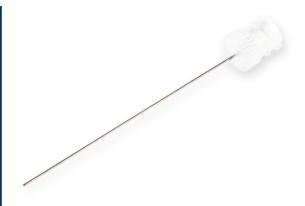
Kel-F hub (KF) needles can be used with Luer Tip (LT) and PTFE Luer Lock (TLL) syringes and connectors. Standard needle length is 2" / 51 mm. Kel-F hub (KF) needles are available in convenient six packs. Custom lengths and point styles are available. These needles are available from 10 - 31 gauge.
