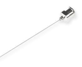
Metal (N) hub needles (nickel plated brass) are compatible with PTFE Luer Lock (TLL) syringes and plastic Luer Tip (LT) or Luer Lock (TLL) connectors. These 304 stainless steel needles are packaged in convenient 6 packs and are available from 10-30 gauge. Custom needle lengths and point styles are available.
