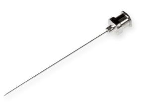
Metal (N) hub needles (nickel plated brass) are compatible with PTFE Luer Lock (TLL) syringes and plastic Luer Tip (LT) or Luer Lock (TLL) connectors. These 304 stainless steel needles are packaged in convenient 6 packs and are available from 10-30 gauge. Custom needle lengths and point styles are available.
