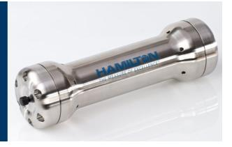
Inherent reversed-phase characteristics make the PRP-1 a rugged, multi-purpose column.
