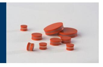
Three Layer Septa is made of preconditioned silicone rubber and is 3.81 mm (0.150 in) thick. The average life of these septa is up to 100 injections with a 26 s gauge needle. The maximum operating temperature is  $200 ^{\circ}$  C.
