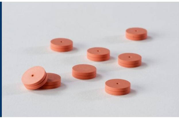
Long Life GC Autosampler Septa are designed for use with GC Autosamplers. The 5, 9, 11 and 11.5 mm diameter Long Life septa are available with a unique pre-pierced center depression to guide the syringe needle to the same injection point, extending septa life, reducing needle bending and eliminates the common type of coring that occurs on the first injection.
