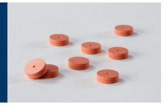
Long Life GC Autosampler Septa are designed for use with GC Autosamplers. The 5, 9, 11 and 11.5 mm diameter Long Life septa are available with a unique pre-pierced center depression to guide the syringe needle to the same injection point, extending septa life, reducing needle bending and eliminates the common type of coring that occurs on the first injection.
