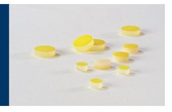
High Temperature Septa is made of preconditioned PTFE/silicone rubber and is 3.175 mm (0.125 in) thick. The average life of these septa is up to 100 injections with a 26 s gauge needle. The maximum operating temperature is  $212 ^{\circ}$  C.
