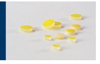
High Temperature Septa is made of preconditioned PTFE/silicone rubber and is 3.175 mm (0.125 in) thick. The average life of these septa is up to 100 injections with a 26s gauge needle. The maximum operating temperature is 212° C.
