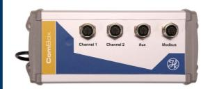
The Cell Density ComBox is a 2-channel USB device that enables the connection of two cell density sensors to the USB port of a Windows PC. The user provided PC must be compatible with the Hamilton cell density software.
