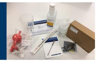
The Validation / Calibration Kit for Incyte contains all material needed for two calibrations and several calibration validation checks for Incyte Sensors, including the permittivity simulator (Ref. 243743), Solution A (Ref. 238988) and Solution B (Ref. 243742).
