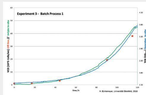
Performance comparison of cell density measurement for the batch set-up.
