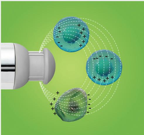
The Incyte is based on capacitance principles. In an alternating electrical field, viable cells behave like small capacitors. The charge from these small capacitors is measured by the sensor and reported as permittivity (capacitance per area).
