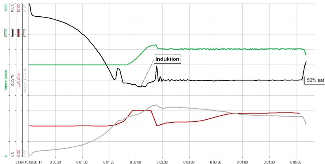
Figure 1: Example of a bioreactor with in-situ process sensors for a microbial fermentation. The chart represents the real-time monitoring of CPPs such as the Dissolved Oxygen as % saturation (signal in black).
