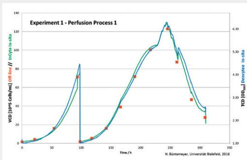
Performance comparison of cell density measurement for the perfusion set-up.
