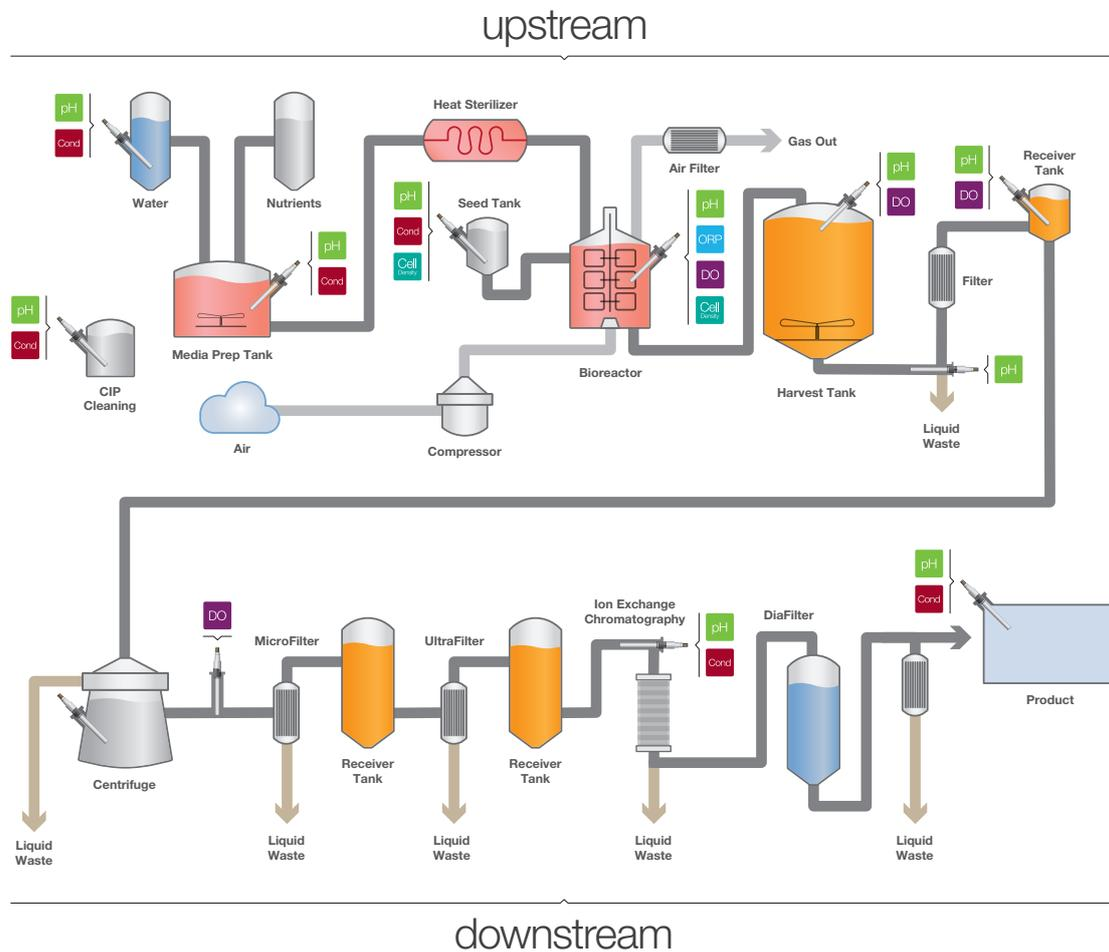
Figure 2: Biopharmaceutical manufacturing process. This map shows the commonly monitored real-time Critical Control Parameters pH in green, ORP in blue, DO in violet, Conductivity in red and the Key Performance Indicator Cell Density in teal.
