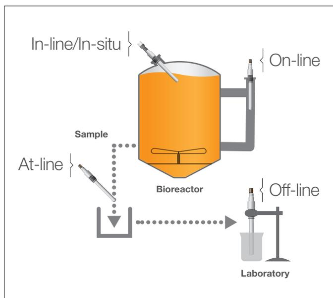
Figure 3: Different methods of process monitoring according to the PAT guidance (2004) & later scientific literature
