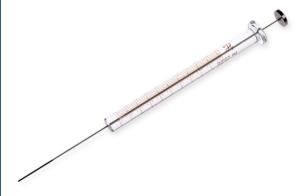
The needles on Thin Layer Chromatography (TLC) syringes are coated from the point for 3/4" with a PTFE-coating. The coating reduces the surface tension between the needle and the liquid making it ideal for reproducible sample spotting.
