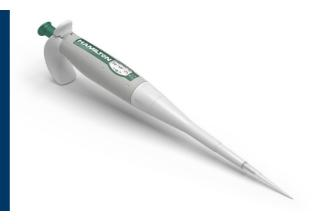
Available in  $0.2\mu$ L - 1 mL, SoftGrip's isolated volume adjustment increases accuracy by removing parallax errors and preventing accidental volume adjustment, thanks to our next-generation dual indicator. Hamilton pipettors boast a slim design that allows for reaching the bottom of narrow tubes without the need for extended-length tips.
