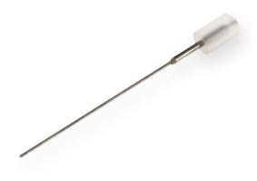
These are replacement needles for the fixed width Gel Loading Syringe. The needles are available in 0.2, 0.3, and 0.4 mm outer diameters. The 0.2 and 0.3 mm needles are jacketed with a thicker gauge needle so only a short distance of the fine gauge needle is exposed.
