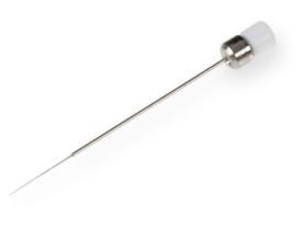
These are replacement needles for the fixed width Gel Loading Syringe. The needles are available in 0.2, 0.3, and 0.4 mm outer diameters. The 0.2 and 0.3 mm needles are jacketed with a thicker gauge needle so only a short distance of the fine gauge needle is exposed.
