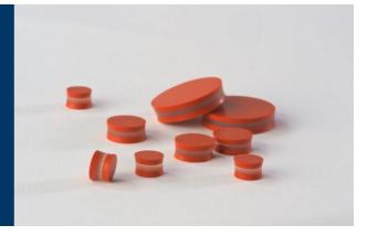
Three Layer Septa is made of preconditioned silicone rubber and is 3.81 mm (0.150 in) thick. The average life of these septa is up to 100 injections with a 26s gauge needle. The maximum operating temperature is 200° C.
