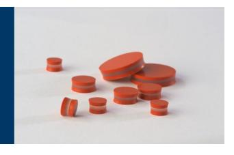
Three Layer Septa is made of preconditioned silicone rubber and is 3.81 mm (0.150 in) thick. The average life of these septa is up to 100 injections with a 26 s gauge needle. The maximum operating temperature is  $200 ^{\circ}$  C.
