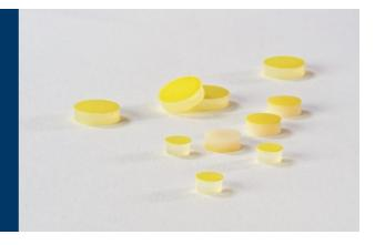
High Temperature Septa is made of preconditioned PTFE/silicone rubber and is 3.175 mm (0.125 in) thick. The average life of these septa is up to 100 injections with a 26 s gauge needle. The maximum operating temperature is  $212 ^{\circ}$  C.
