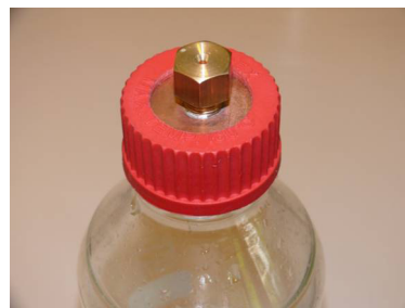
Figure 2: 1L glass bottle with a septum in the screw cap used for the HS GC analysis of a mixture of halogenated hydrocarbons.
