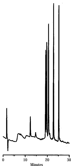
Figure 19 Five Peptide Standards HxSil C8, 4.6 x 150 mm, 5 µm (P/N 79102)
