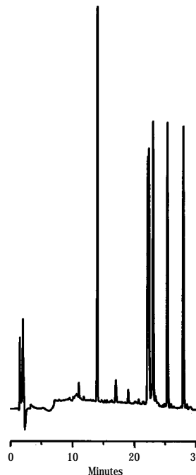
Figure 18 Five Peptide Standards HxSil C18, 4.6 x 150 mm, 5 µm (P/N 79868)
