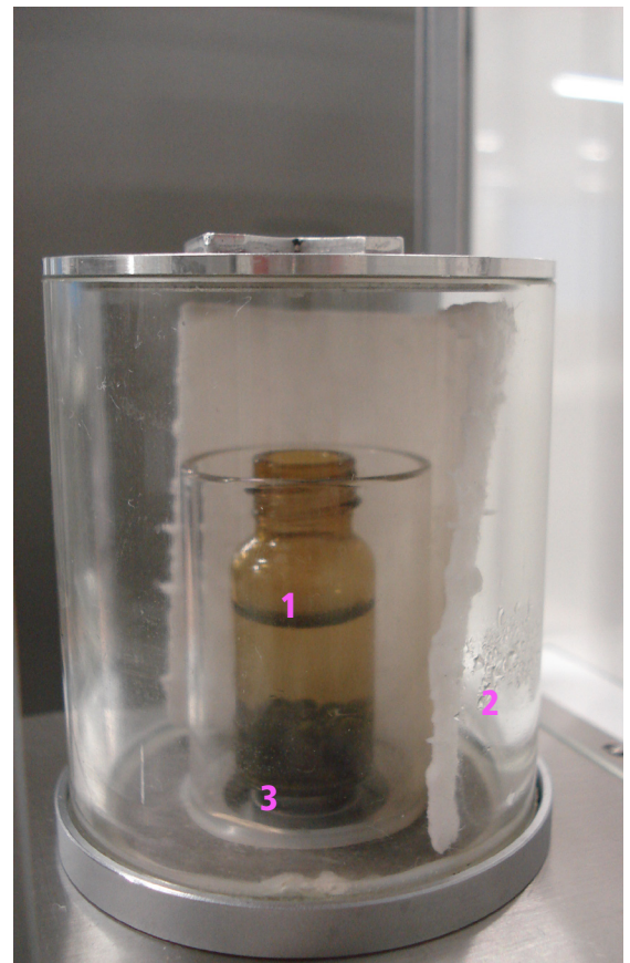
Figure 1: Sample aspiration chamber 1: Sample vessel with deionized water 2: Evaporation protection 3: Deionized water at the bottom of the evaporation protection
