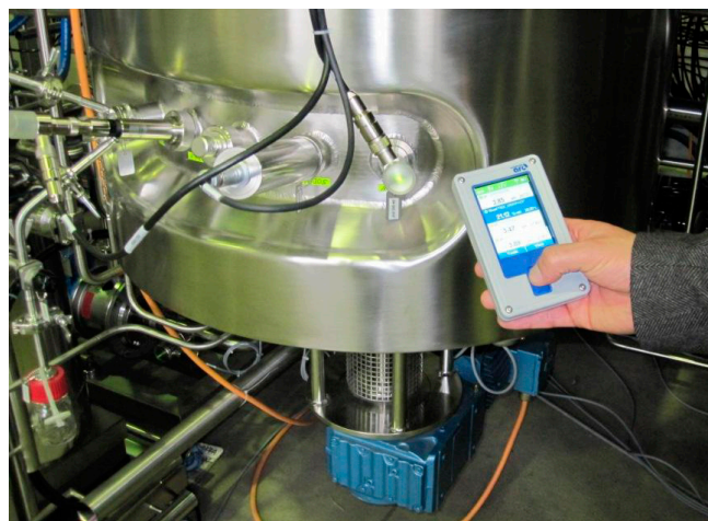
Figure 3: ARC sensor operation with ARC View Handheld at main fermenter
