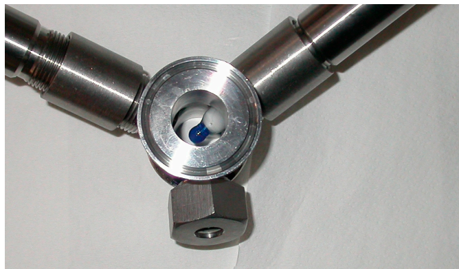
Figure 2: DO sensor (left), pH sensor (right) and sample port (in front) mounted between static mixer modules of the PFR
